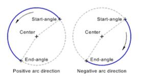
The eventual appearance of the reference circle part is shown during entry, and changes if the arc direction is changed during entry.
