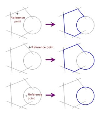
The effect of the reference point can be explained (simply) as follows: Imagine emptying a can of paint at the reference point. The paint spreads out in all directions until it reaches an object. The result is one area which is covered in paint, and one area which is not. The boundary between these two areas is the outline of the newly-generated surface.
