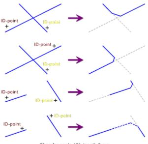
Chamfer angle 45°, length 3 mm
