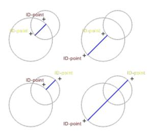
After determining the distance to be measured, the position of the dimension line and dimension text must be specified. To do this, several points have to be entered. How many, and which, points have to be
