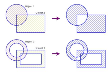
The areas of the objects shown hatched are hatched or filled if the relevant object is hatched or filled. The effects of this combination can be expressed as: (Object 1 - Object 2)  $\times$  (Object 2 - Object 1).
