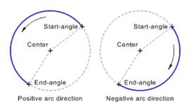
The appearance of the circular arc is shown during input, and changes if the current arc direction is changed.
