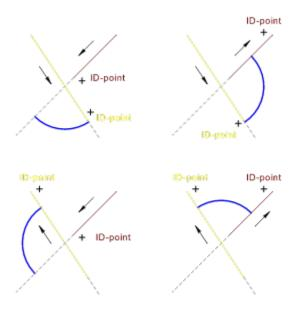
The position of the ID point with reference to each leg shows which angle is measured.
