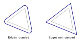
Because of the definition of equidistants (the same distance from all points), all corners must theoretically be rounded. In many cases this is not required, and therefore this procedure is provided.
