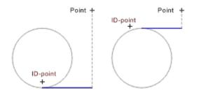
After identifying the object, a straight line appears which runs horizontally and is tangent to the identified object. This line is referred to as the "Reference Straight Line".
