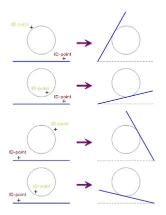
If the trim object is a circle or ellipse part, then the arc end angle closer to the ID point is changed (see graphic).
