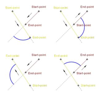
After entering the legs of the angle to be measured, the position of the dimension line and the dimension text must be specified. To do this, several points have to be entered. How many, and which, points have to be entered, depends on the specified dimension parameters.
